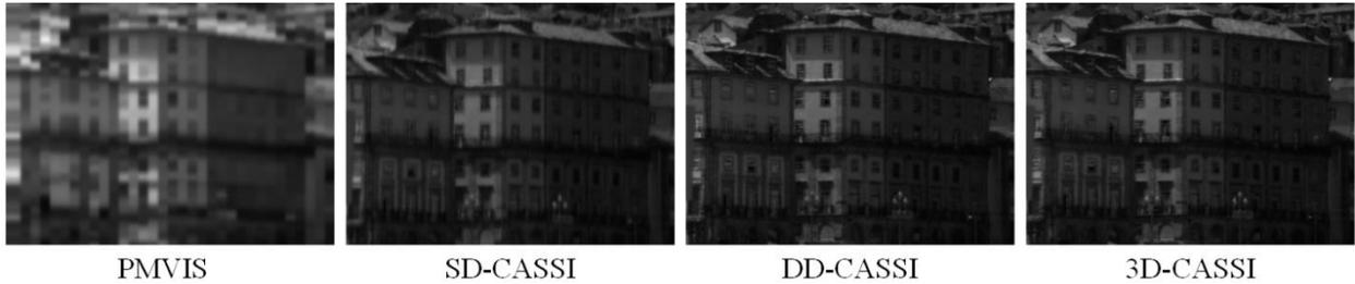
Figure 9. Comparison of reconstructed results for the four under-sampling systems. All the results are shown at the 610nm channel. (PMVIS PSNR = 16.6845db, SD-CASSI PSNR = 18.0859db, DD-CASSI PSNR = 29.8178db, 3D-CASSI PSNR = 32.5659db)
